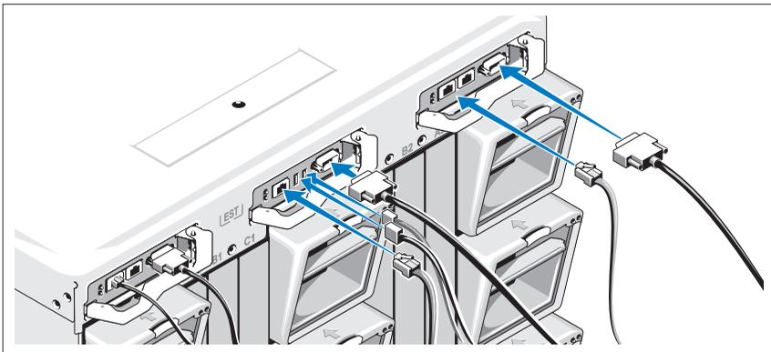
Connect the serial cable and network cable(s) from the management system to the CMC module. If a second, optional CMC module is installed, connect it as well.
